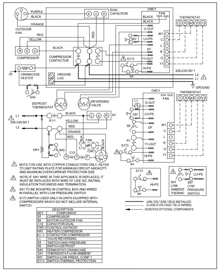
Figure 14. Typical Unit Wiring Diagram
